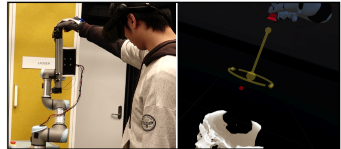
Fig. 18. Robotic arm holding the rotary encoder for rotational interactions according to hand position (left). Select the rotary control in the virtual world and rotate the virtual skeleton around that axis (right).
