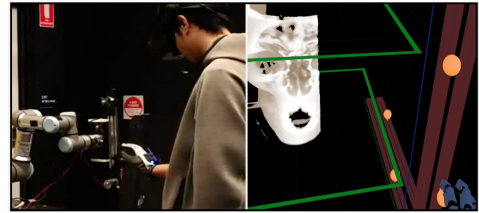
Fig. 17. One robotic arm and one mounted slider represents multiple slider controls and reaches to the required position according to hand position (left). Select a slicing plane of a skeleton in the virtual world and move among in three axis direction (right).
