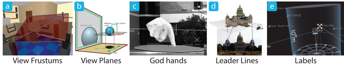
Fig. 8. Several examples of Links on WiMs: (a) a view frustum showing the viewer’s position and orientation in the scene [34], (b) a slicing plane controlling the viewable space [11], (c) a god hand indicating where a viewer is pointing in the environment [43], (d) leader lines connecting components of the replica to their real twin [45], (e) labels identifying components of the WiM [26]. Images reused with permission.
