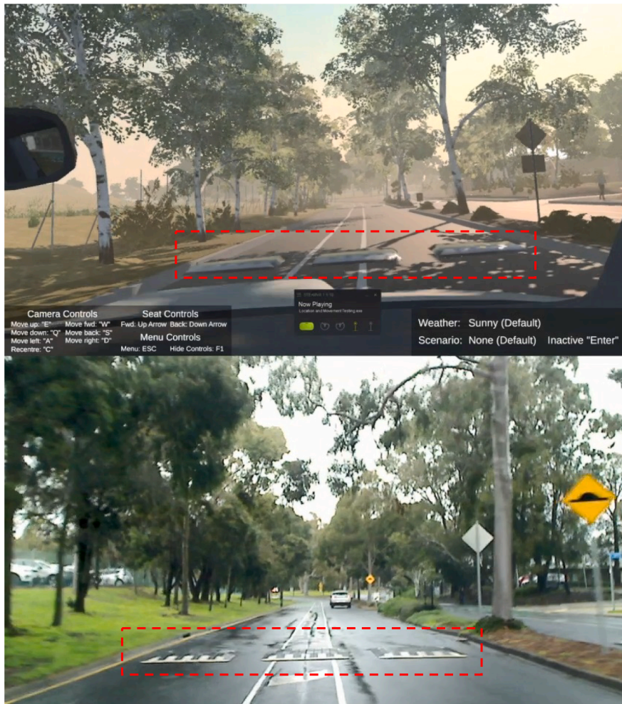
Fig. 6. Views of speed humps in both the virtual (upper) and real worlds (lower) at the same time.
