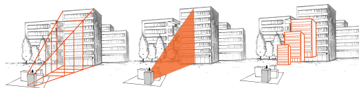
Fig. 4. Link geometries with the size of real-world targets: 3D tunnel (left), 2D surface (center), and moving mesh (right).
